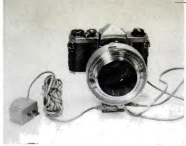
Plug-in jacks give choice of full, half or quarter output. Adapter for a.c. is shown in photo at right
